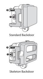
**2** Unhook the buckle from the housing to open the backdoor.
