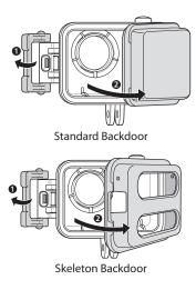
**3** Insert the camera into the waterproof housing.
