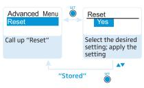
When resetting the settings made in the operating menu, only the selected settings for the pilot tone and for the frequency banks "U1" to "U6" remain unchanged. For an overview of the factory-preset default settings, refer to the enclosed frequency information sheet.
