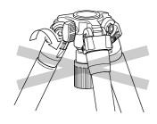
Do not turn the Center column stopper while pulling out the Center column. The internal parts may be damaged.
