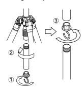
Remove the Center column base stopper, and then remove the Lower part of Center column.
