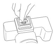
Align the length of the platform along the base of the camera body, and securely tighten the mounting wing nut.
