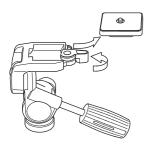
Remove the quick release platform turning the lock lever.
