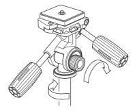
Set the new head, or accessory on the tripod's threaded post, and turn clockwise until it comes to a stop. Tighten the panning lock knob and turn clockwise slightly more.
