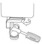
When you fix this quick release platform to pan head, the quick release lock lever will return to the original position automatically. We, however, recommend you to tighten this lever more to secure the fixing.
