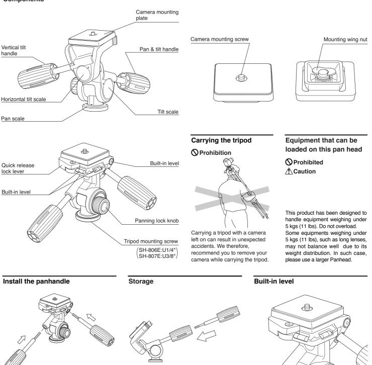
Panhandle are installed as shown. There is not difference in length between the panhandle. Panhandle is installed in both side.
