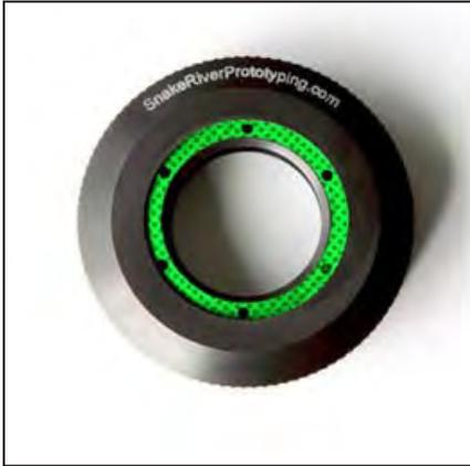
6. Use a toothpick to apply sealant on only the surface that contains the screw holes (see the highlighted area in the figure to the left). Apply sealant especially along the outside edge of this surface so that it fills in the corner between the surface with the screw holes and the top most surface. Also, place a dab of sealant into each of the screw holes. Be careful not to get any sealant on the inner beveled edge which will come in contact with the GoPro OEM lens in the next step.
