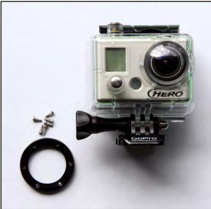
4. Wipe the OEM lens clean if necessary, then place it on the rubber seal. Set the partially assembled unit to the side for now.
