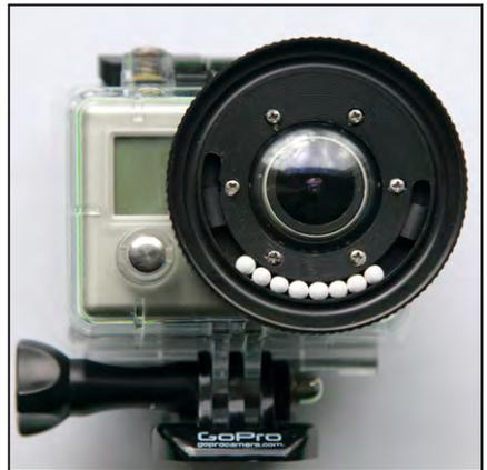
2. Move the desiccant balls into the position shown. Insert two rubber stoppers into the lollipop groove, one on each side of the desiccant balls.
