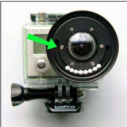
1. Insert eight desiccant balls into the lollipop groove using the entry hole shown in the above figure. Place your thumb over the entry hole, turn the housing upside down, and shake the whole unit. Replace any balls that fall out with larger ones.
