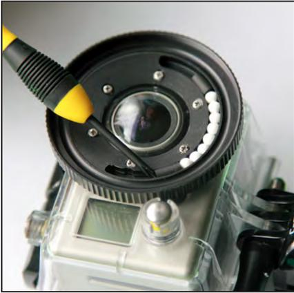
3. Use the Phillips screwdriver to move the rubber stoppers into contact with the desiccant balls so that the balls stay centered at the bottom of the lollipop groove.
