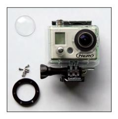
3. Should the OEM lens and/or rubber seal come off, first install the rubber seal with the sharp rubber lip facing away from the housing.
