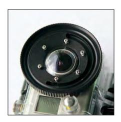
8. Install the screws loosely. Only turn each screw a few turns until all screws are installed. Once all the screws have been started, turn each screw until its head comes in contact with the BlurFix.
