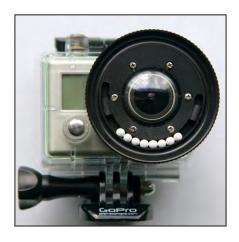
2. Move the desiccant balls into the position shown. Insert two rubber stoppers into the lollipop groove, one on each side of the desiccant balls.
