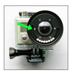
I. Insert eight desiccant balls into the lollipop groove using the entry hole shown in the above figure. Place your thumb over the entry hole, turn the housing upside down, and shake the whole unit. Replace any balls that fall out with larger ones.
