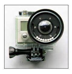
2. Place the o-ring in the o-ring groove.
