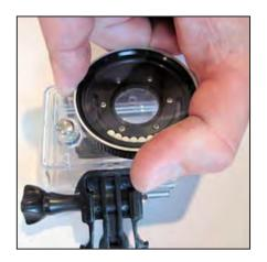
3. Gently thread the filter onto the BlurFix. Holding the housing in your left hand, wrap your right thumb around the filter as shown. Using your thumb, index finger, and the side of your middle finger to maximize your surface contact with the filter, tighten the filter down allowing it to slip in your fingers. Repeat several times. Look through the filter at the o-ring. You should see a dark black line where the filter seals against the o-ring.
