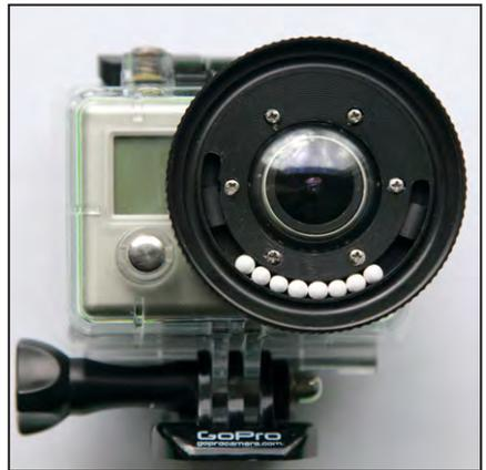
1. Insert eight desiccant balls into the lollipop groove using the entry hole shown in the above figure. Place your thumb over the entry hole, turn the housing upside down, and shake the whole unit. Replace any balls that fall out with larger ones.
