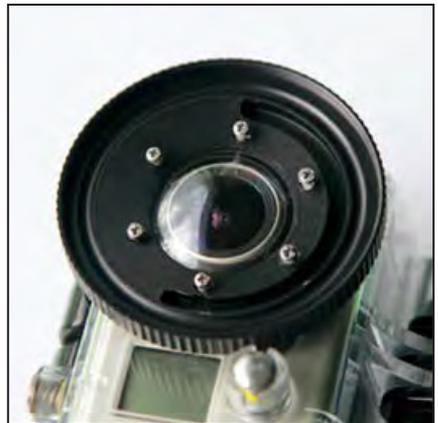
8. Install the screws loosely. Only turn each screw a few turns until all screws are installed. Once all the screws have been started, turn each screw until its head comes in contact with the BlurFix. Do not tighten yet.
