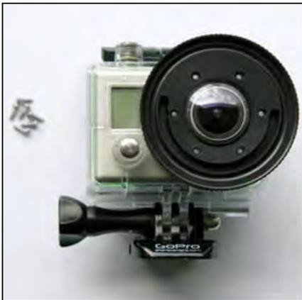
7. Mount the BlurFix onto the housing so that the desiccant groove is at the bottom of the GoPro. Line up the screw holes. Place the GoPro housing on its back as pictured above and press the BlurFix firmly onto the housing.
