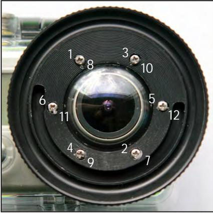
9. Tighten the screws according to the pattern on the left. Repeat the pattern until all screws are snug. **DO NOT** over-tighten as you will strip out the screw holes in the case. Open the back of the GoPro case and look through the housing to verify that the silicone has formed a seal between the GoPro housing and BlurFix.
