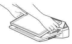
The magnet locks will lock the display into place.
