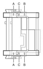
A and C: Sets the stand towards the back. B and C: Sets the stand towards the front.
