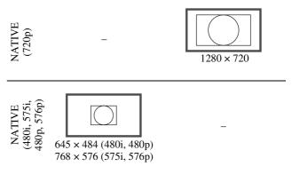
To display in 4:3 aspect ratio, images are adjusted horizontally with scale handling.
