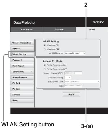
**2** Enable or disable the radio wave output of USB wireless LAN module.
