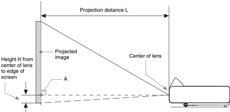
\* The number will be minus when the bottom of the projected image is lower than A.
