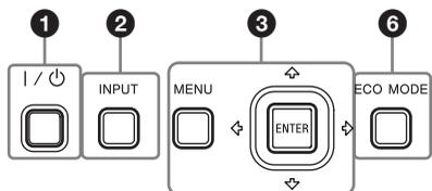
**1 Turning on the power/Going to standby mode**
