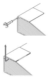
3 Loosen the three screws on the lamp
