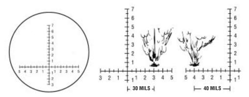
Fire corrections can be made by viewing the impact area and determining angular corrections by use of the left or right horizontal reticle scale.
