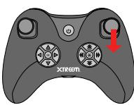
**Turbo:** The Turbo button makes your helicopter move forwards/backwards faster by increasing the speed of the tail rotor. Press once to enable turbo mode. To return to normal speed, press again.
