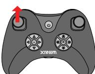
**Moving up and down:** The helicopter moves up and down by varying the speed of its main rotors (those two big things that spin). You can control how fast these spin by using the left stick on the controller. Pushing the stick up will increase the throttle.
