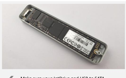
Make sure your JetDrive and USB to SATA adapter is laying flat inside the enclosure
