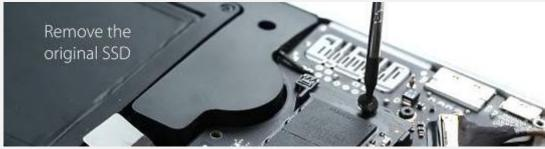
Use the included P5 screwdriver to remove the back cover and the T5 screwdriver to remove the screw from the rear of the SSD. Carefully remove the original SSD and insert your JetDrive. Replace all screws to finish the installation
