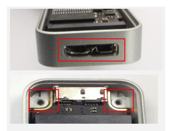
Make sure the USB connector is located correctly in the opening as shown.
