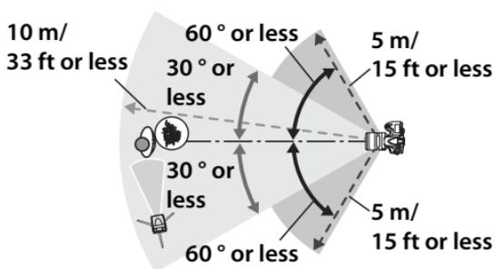
Wireless remote sensors on flash units should face camera.
