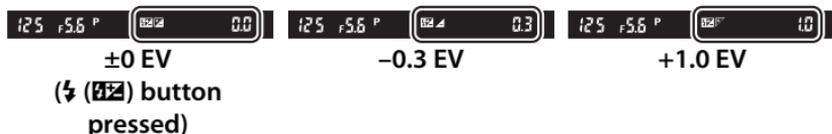
At values other than  $\pm 0.0$ , a **⚡ (FLC)** icon will be displayed in the control panel and viewfinder after you release the **⚡ (FLC)** button. The current value for flash compensation can be confirmed by pressing the **⚡ (FLC)** button.
