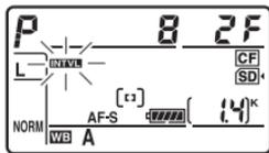
To view current interval timer settings, select **Interval timer shooting** between shots. While interval timer photography is in progress, the interval timer menu will show the starting time, the shooting interval, and the number of intervals and shots remaining. None of these items can be changed while interval timer photography is in progress.
