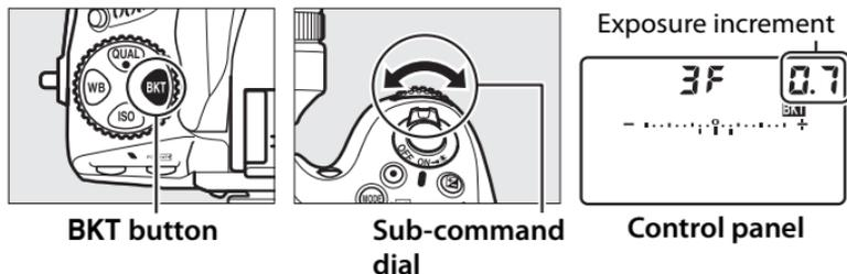
At default settings, the size of the increment can be chosen from  $\frac{1}{3}$ ,  $\frac{2}{3}$ , and 1 EV. The bracketing programs with an increment of  $\frac{1}{3}$  EV are listed below.
