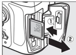
**CompactFlash memory cards:** Press the eject button (①) to partially eject the card (②). The memory card can then be removed by hand. Do not push on the memory card while pressing the eject button. Failure to observe this precaution could damage the camera or memory card.
