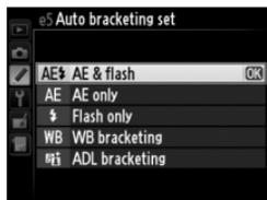
Choose **AE & flash** to vary both exposure and flash level, **AE only** to vary only exposure, or **Flash only** to vary only flash level.
