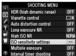
Note that ISO sensitivity can not be adjusted from the shooting menu in movie live view. In exposure mode **M**, ISO sensitivity can however be adjusted using the **ISO** button and main command dial (☰ 109).
