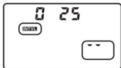
To view current time-lapse photography settings, press the **MENU** button between shots. While time-lapse photography is in progress, the time-lapse photography menu will show the interval and the time remaining. These settings can not be changed while time-lapse photography is in progress, nor can pictures be played back or other menu settings adjusted.
