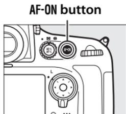
The focus point will blink green while the camera focuses. If the camera is able to focus, the focus point will be displayed in green; if the camera is unable to focus, the focus point will blink red (note that pictures can be taken even when the focus point blinks red; check focus in the monitor before shooting). Exposure can be locked by pressing the **AE-L/AF-L** button (□ 128); focus locks while the shutter-release button is pressed halfway.
