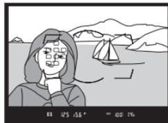
AF-area mode can be selected by pressing the AF-mode button and rotating the sub-command dial until the desired setting is displayed in the viewfinder and control panel.
