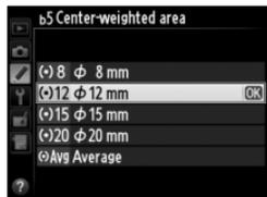
Note that unless **Average** is selected, the diameter is fixed at 12 mm when a non-CPU lens is used, regardless of the setting selected for **Non-CPU lens data** in the setup menu (📖 212). When **Average** is selected, the average of the entire frame will be used for both CPU and non-CPU lenses.
