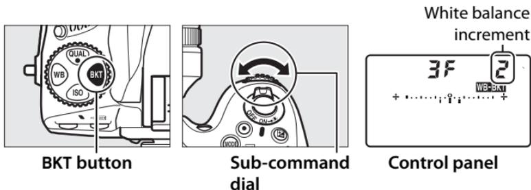
Choose from increments of 1 (5 mired), 2 (10 mired), or 3 (15 mired). Higher **B** values correspond to increased amounts of blue, higher **A** values to increased amounts of amber (□ 149). The bracketing programs with an increment of 1 are listed below.
