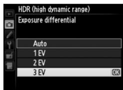
choosing a value higher than required may not produce the desired results; if **Auto** is selected, the camera will automatically adjust exposure to suit the scene.
