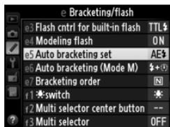
To display the menus, press the MENU button. Select Custom Setting e5 (**Auto bracketing set**) in the Custom Settings menu, highlight an option, and press OK.
