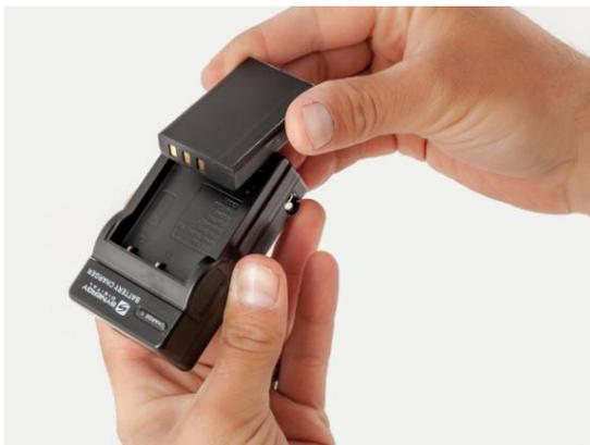
3. Install the NP-120 battery included with the STREAM into the battery mount.
