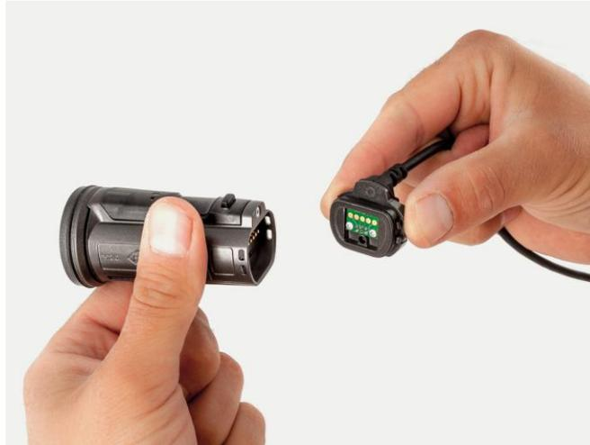
**Set up the V.I.O. STREAM with a Battery end cap and mount**
