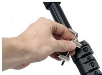
Should the leg clamps become loose over time, use the supplied socket wrench to tighten them.
