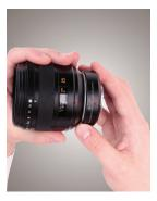
6. Align the red mark on the lens adapter with the red lens attachment mark on the camera and slowly rotate the adapter and lens clockwise until it clicks into place on the camera.
