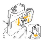
4. To prevent loss, place the camera battery chamber cover in the BG-C8 battery chamber holder, as indicated above. Swing the battery chamber cover shut so that it locks into place
