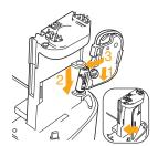
4. To prevent loss, place the camera battery chamber cover into the BG-C9 battery chamber holder as indicated above. Swing the battery chamber cover shut so that it locks into place.
