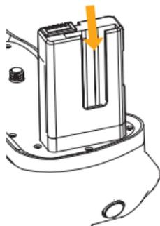
3. Slide the camera battery chamber door into the BG-N13 chamber door holder in order to avoid loss.
