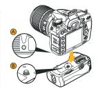
5. Connect the BG-N4.2 grip to the camera, while aligning the camera's tripod socket (A) with the grip's mounting screw (B).
