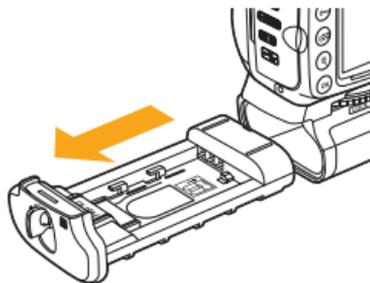
2. Remove the battery holder from the BG-N8 grip. The EN-EL3e battery holder comes pre-installed when shipped.
