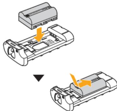
3. Nikon EN-EL3e Batteries: Matching the indentations on the battery with the EN-EL3e holder, press the battery down and slide it in the direction of the arrow until the power terminals click into place.
