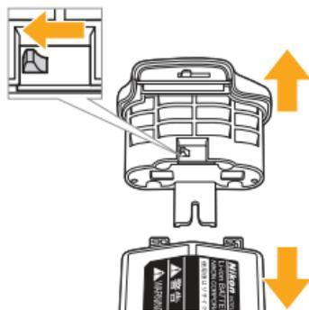
2. BC-N1 Holder: Slide the battery release in the direction indicated by the arrow and remove the battery.
