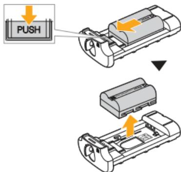
1. EN-EL3e Holder: While pressing and holding the PUSH button on the holder, slide the battery toward the button and lift up to remove.
