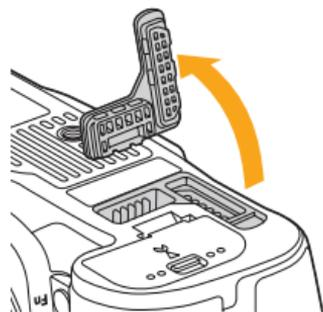
3. The contacts for the BG-N8 are on the bottom of the camera where they are protected by a contact cover. Remove the contact cover before mounting the grip.
