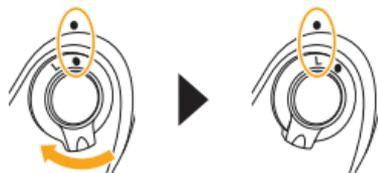
1. Ensure that the power is turned off on the camera and that the Control Lock on the BG-N8 is in the **L** position before attaching the grip.
