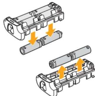
3. AA Holder: Remove the batteries one row at a time (as shown). Ensure that the batteries do not drop during this process.
