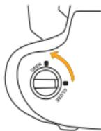
2. Rotate the dial on the battery chamber door to OPEN position, and the door will open up.
