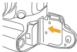
5. Slide the battery tray into the battery chamber until it locks into place. Close the battery chamber door and lock it by rotating the dial to CLOSE position.
