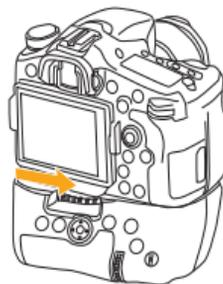
5. Rotate the attachment wheel in the direction shown by the arrow until it is firmly tightened.
