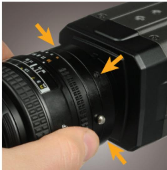
4. If desired, you can re-align the lens to a specific position. To re-align the lens, use a 2 mm flat-head screwdriver to loosen the three screws on the lens mount. Rotate the lens to the desired position, and tighten the three screws.
