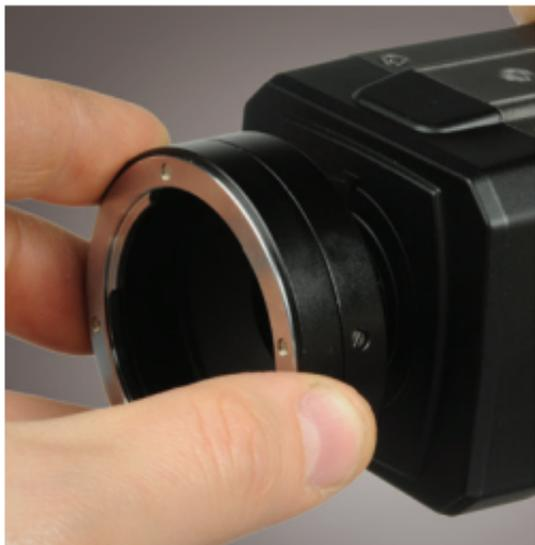
**3.** Rotate the lens adapter to remove.
