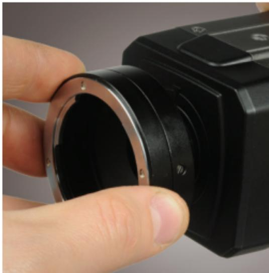
**1.** Rotate the lens adapter clockwise onto the camera until it is secure.
