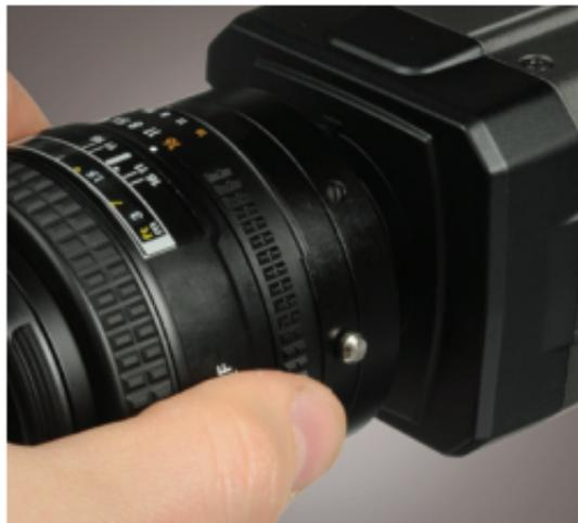
**2.** Rotate the lens to release.
