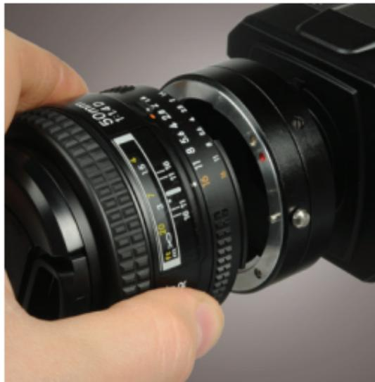
**2.** Line up the alignment dots on the lens and the lens adapter.
