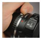
3. Lift and hold the release pin on the lens adapter.
