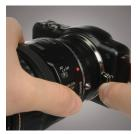
Press the lens release button on the camera.
