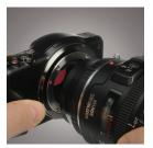
**3.** Line up the alignment dots on the lens adapter and the camera.
