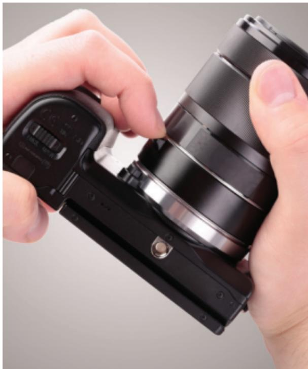
2. Press the camera's lens release button and remove the tube as you would a normal lens.
