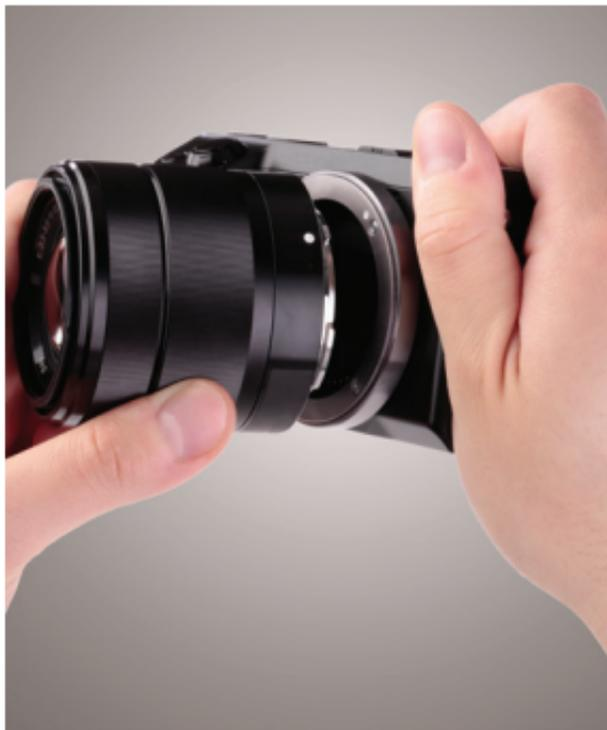
2. Align the Vello extension tube to the camera's lens mount. The extension tube will mount in exactly the same manner as a standard lens. Make sure to align the alignment dot on the tube with the circular alignment mark on your camera.
