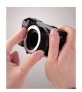
3. Mount your lens onto the extension tube in exactly the same manner as you would mount it on the camera.
