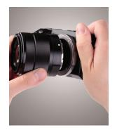
Align the Vello extension tube to the camera's lens mount. The extension tube will mount in exactly the same manner as a standard lens. Make sure to align the alignment dot on the tube with the circular alignment mark on your camera.
