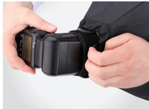
2. Continue rocking the softbox forward until it disengages fully from the touch fastener cinch strap on the head of the portable flash.
