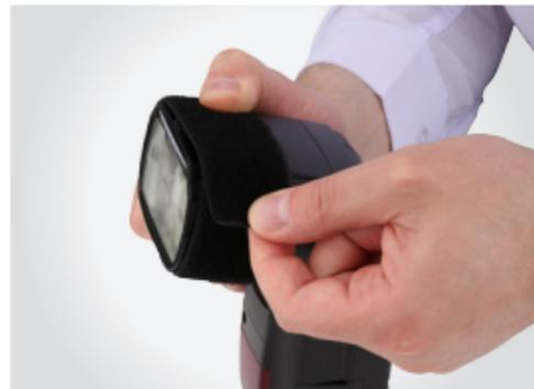
2. Place the bottom of the flash head against the bottom mounting tab of the softbox, just about halfway into the softbox.
