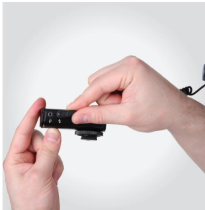
5. Plug the 3.5 mm side of the cable into the studio flash sync jack.
