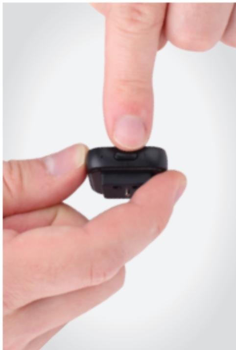
5. Both the transmitter and the receiver should now be paired. To verify communication, press the transmitter's pairing/test button. The indicator light on the receiver will register one quick blink.
