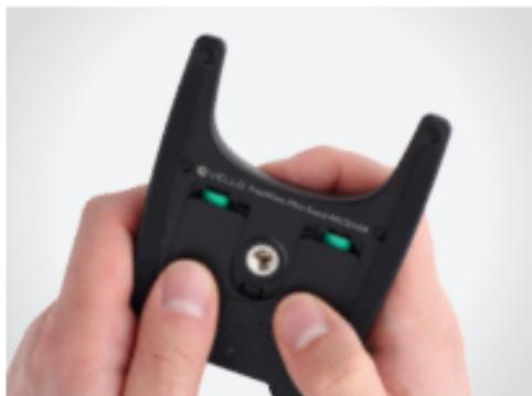
8. Reattach the battery compartment cover for each receiver.
