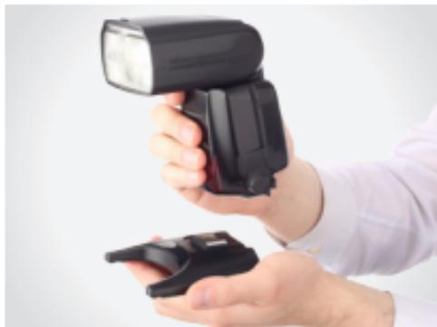
10. Turn the flash on and press the pairing/test button on each transmitter. Each of the transmitters should fire the flash unit.
