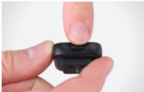
3. Secure the flash by engaging its locking mechanism.
