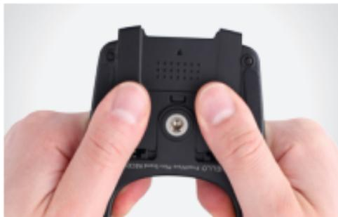
3. Press the recessed transmitter code set button on the receiver. Use a pin-like object that will fit into the recessed hole.
