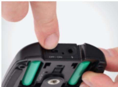
2. Press the recessed transmitter code set button. Use a pin-like object that will fit into the recessed hole.
