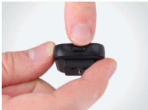
5. Both the transmitter and the receiver should now be paired. To verify communication, press the transmitter's pairing/test button. The indicator light on the receiver will register one quick blink.
