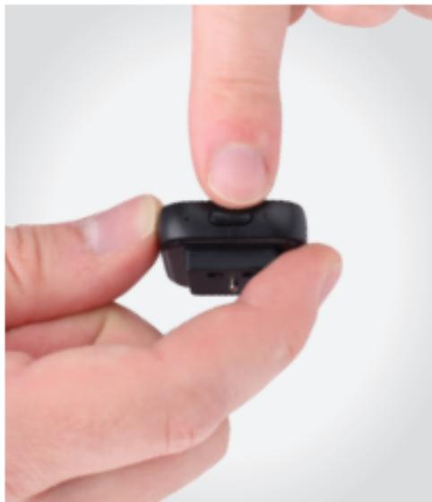
6. In these 5 seconds, you will need to press the pairing/test button on the next transmitter, and so on for the remaining transmitters. The receiver's status indicator light will blink twice and then flash repeatedly again for 5 seconds after each transmitter has been paired.
