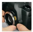
2. Press and hold the lens release button on the camera. Rotate the lens adapter counterclockwise to release.
