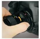
2. Rotate the lens counterclockwise to release.
