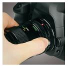
Press and hold the release button on the lens.
