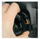
Rotate the collar on the lens adapter in the direction of the arrow to the LOCK position.
