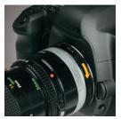
Rotate the collar on the lens adapter in the direction of the arrow to the LOCK position.
