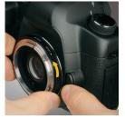
Press and hold the lens release button on the camera. Rotate the lens adapter counterclockwise to release. For Micro Four-Thirds (MFT) cameras, enable the "Shoot without Lens" function in the menu of the camera.
