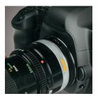
**4.** Rotate the locking collar on the lens clockwise until it is secure.
