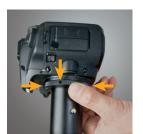
5. If desired, you can re-align the lens to a specific position. To re-align the lens, use a 2 mm flat-head screwdriver to loosen the three screws on the lens mount. Rotate the lens to the desired position, and tighten the three screws.
