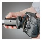
Line up the alignment dots on the lens adapter and camera. Rotate the assembly until it locks.
