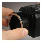
1. Rotate the lens adapter clockwise onto the camera until it is secure.
