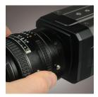
3. Rotate the lens until it locks into place.
