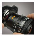
Line up the alignment dots on the lens adapter and the camera. Rotate the lens assembly clockwise until it locks into place.
