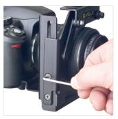
Loosen the two screws on the side of the upright arm.
