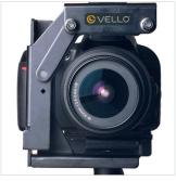
Adjust the bracket's position. The center of the lens should align with the \$\ightrigorightarrow\$ shaped hole in the bracket.
