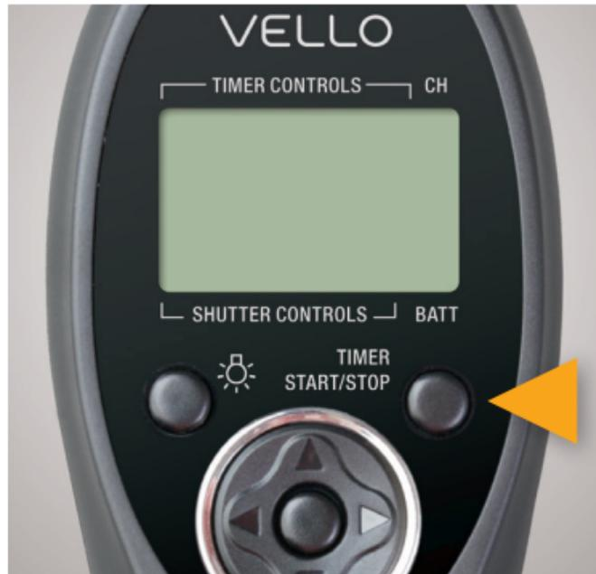
*Once you've set up your Timer Controls, press the Timer Start/Stop button to begin the countdowns and exposures.*
