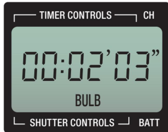
*In bulb mode, the screen will display the seconds of your exposure.*
