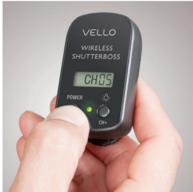
***Press and hold the power button for two seconds to power up the receiver. The LED will blink green while the device is on.***
