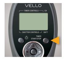
Once you've set up your Timer Controls, press the Timer Start/Stop button to begin the countdowns and exposures.
