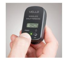
Press and hold the power button for two seconds to power up the receiver. The LED will blink green while the device is on.
