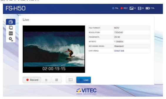
The Live, Record and Snapshot features (and button activity) are available as long as a video input signal is detected.
