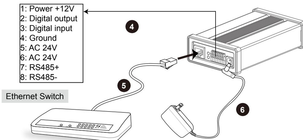
There are several ways to set up the video server over the Internet. The first way is to set up the video server behind a router. The second way is to utilize a static IP. The third way is to use PPPoE.
