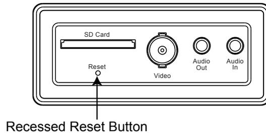
The reset button is used to reset the system or restore the factory default settings. Sometimes resetting the system can return the video server to normal operation. If the system problems remain after reset, restore the factory settings and install again.
