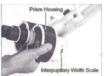
Adjust the interpupillary width to your eyes by rotating both the prism housings equally. Look at a distant object through the eyepieces and move the two halves of the prism housings until the circles of field of view becomes one completely. Insert 31.7mm (1.25") telescope eyepieces of the same focal length into each of the eyepiece holders.
