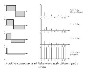
The first thing you probably observe is that the lower part of the wave has a narrower excursion. This is because the energy of the wider pulse is higher than the one of the narrower pulse. If this were not compensated, the overall signal would have an unwanted DC offset.
