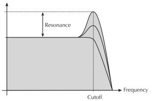
If the resonance is raised to a great extent, then the filter will begin self-oscillation, i.e. the filter generates an audible sine wave even when it does not receive an incoming signal.
