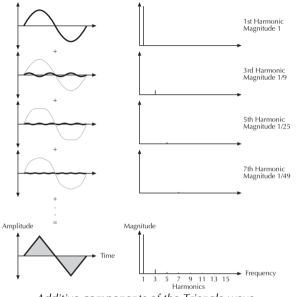
Additive components of the Triangle wave
