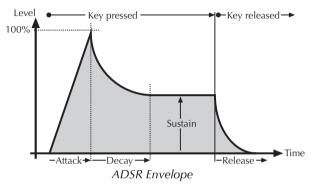
The envelope is started by pressing a key. It ascends to its maximum value at the rate determined by the **Attack** parameter. It then descends at the rate determined by the **Decay** value until it reaches the predetermined **Sustain** value. It remains at this value until the key is released. The envelope then descends to zero at the rate determined by the **Release** parameter.
