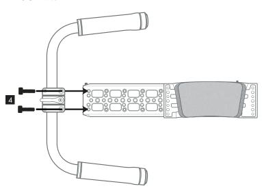
3. With SIDE A facing SAFETY LATCH, align DOVETAIL over SHOULDER PAD as shown below, select 1/4-20x3/8 SOCKET CAPS, tighten with allen wrench
