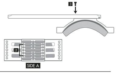
5. Loosen **THUMB SCREW** to adjust **HANDLE BAR** to desired position
