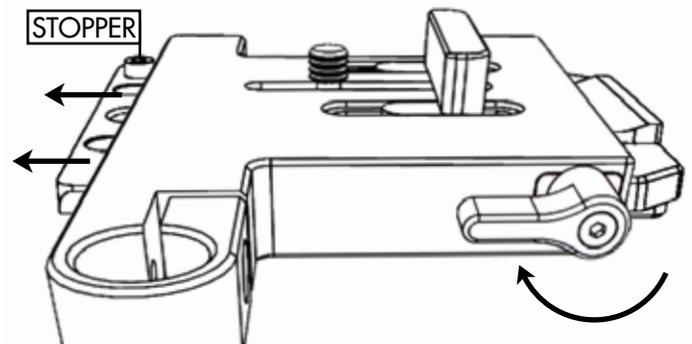
Push **BASE** until contact is made with **STOPPER** before tightening thumbscrew.
