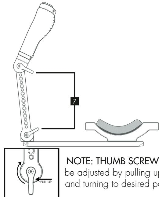
**NOTE: THUMB SCREWS** can be adjusted by pulling upward and turning to desired position
