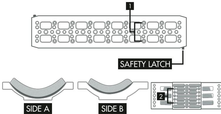
3. With **SIDE A** facing **SAFETY LATCH**, align **DOVETAIL** over **SHOULDER PAD** as shown below, select **1/4-20x3/8 SOCKET CAPS**, tighten with allen wrench
