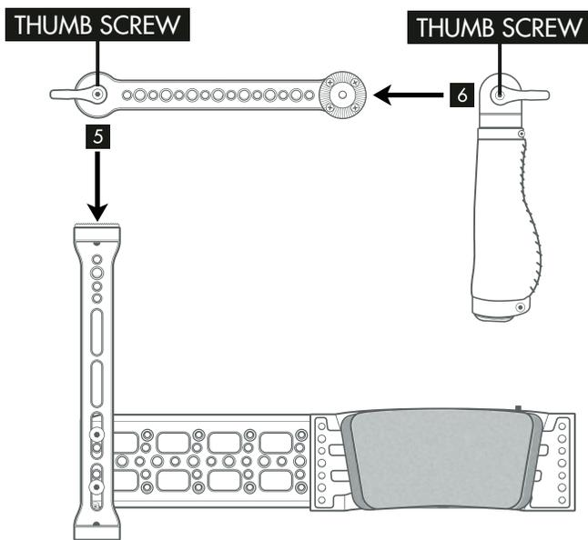
7. Loosen **THUMB SCREWS** to adjust **HANDLES** and **ROSETTE ARMS** to desired position
