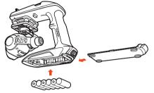
Slide the battery cover / door upward with slight force and inspect the AA battery compartment.
