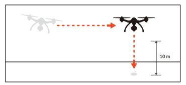
**B)** When flying lower than 33 feet (10 meters) TYPHOON will climb to 33 feet (10 meters) while flying back to the home point, then will descend vertically until it lands.
