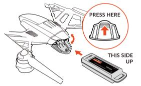
**STEP 1**) Push the area at the top of the battery door to release the latch/lock, and then open the door.
