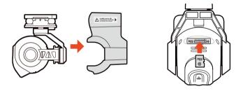
**Step 1)** Remove the cover/lock from the rear of the CGO2+ by carefully sliding it backward.
